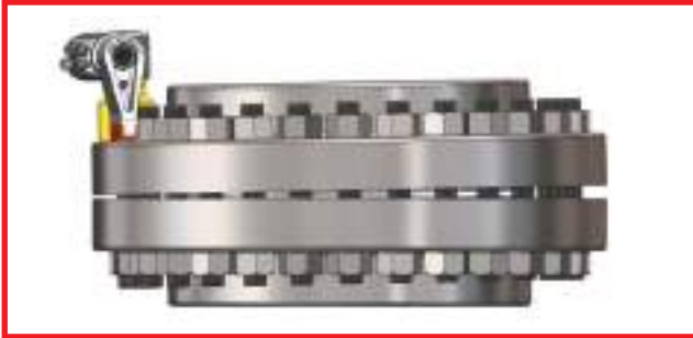
Uneven load using one tool
